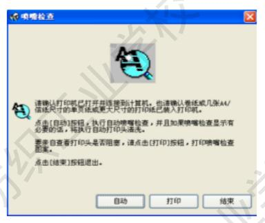
Click the button of "printing", and the printer shall automatically print the pattern on the papers which are placed on the printing platform. According to the printed pattern, it can be judged whether the nozzle is unobstructed.
